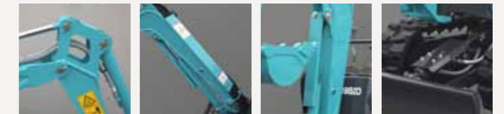
Bucket cylinder hose inside the arm
