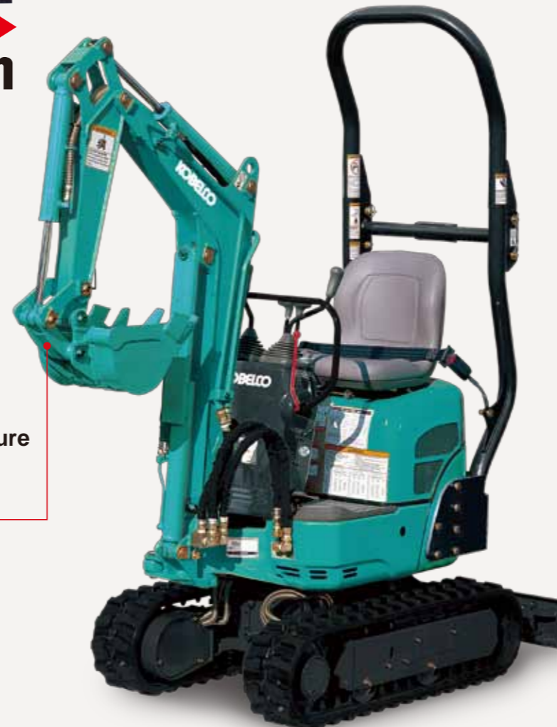
Bucket cylinder hose inside the arm
