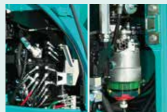
Control valve/water separator tank/air cleaner
