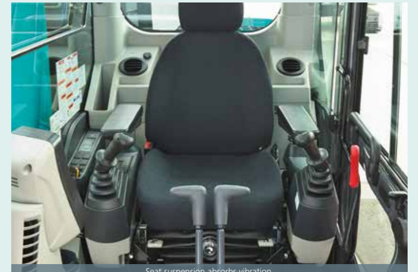
Seat suspension absorbs vibration
