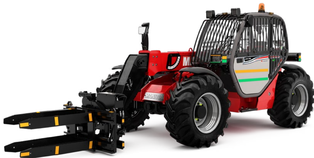
Machine on tyres with forks Stability norm ISO 22915-14
