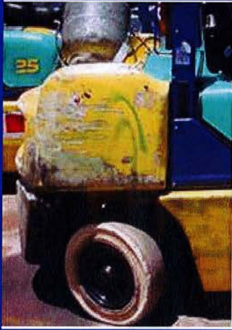
x Unacceptable paint damage
