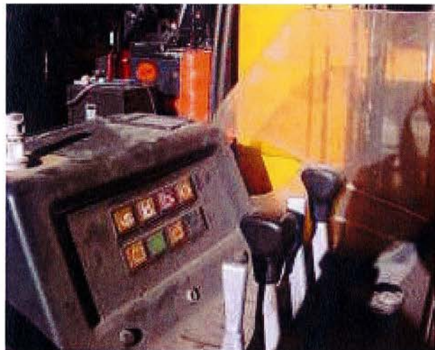
x Unacceptable customer damage. Cracked and broken guard, missing knobs.
