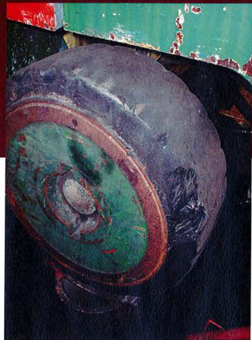
x Unacceptable - Tyre cut
