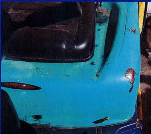
√ Acceptable wear and tear. This paint has worn off from the driver entering and exiting the machine. The paint rubbing near the seat caused by legs and hands. When considering the age and hours of the machine is acceptable wear and tear.
