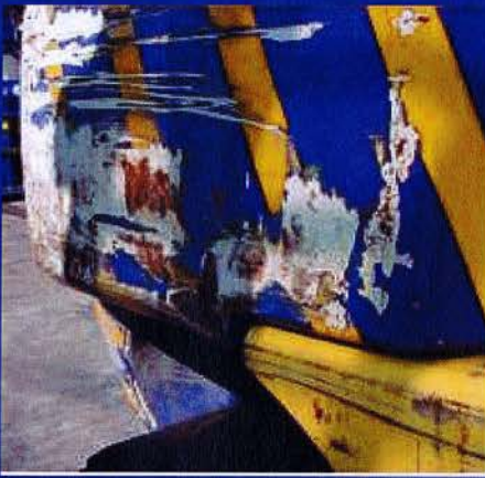
x Unacceptable paint damage
